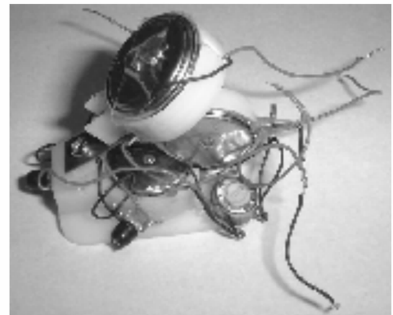
Fig. 12 Resonant hopping locomotion mechanism with optical sensors
