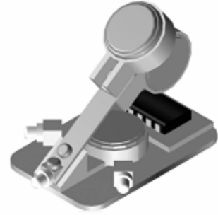
Fig. 8 Module of the resonant hopping locomotion mechanism with optical sensors.
