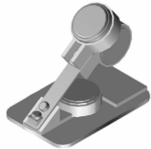
Fig. 7 Module of the resonant hopping locomotion mechanism
