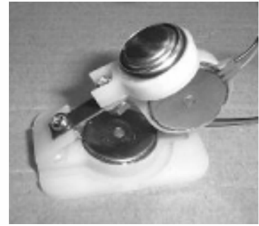
Fig. 11 Resonant hopping locomotion mechanism
